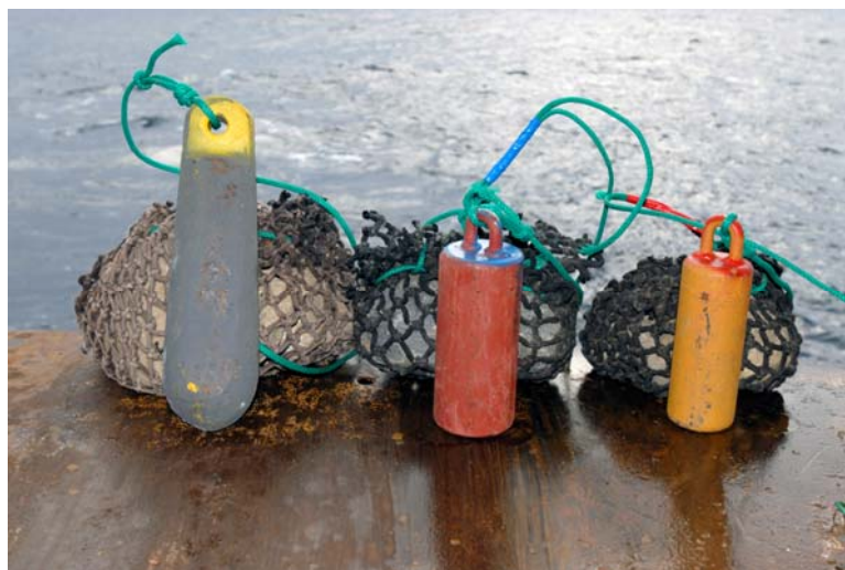
Figure 2. Examples of rock weights (rear) and steel weights used in the experiment. Also shown is the difference in shape between the steel weights produced from a mould (left) and cut from steel rod. Weights from left to right are 8 kg, 6 kg and 4 kg.
