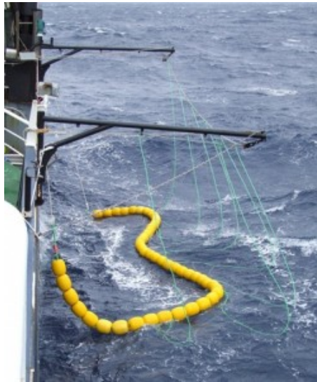
Figure 3: Photograph showing an example of a Bird Exclusion Device (BED) in action.
